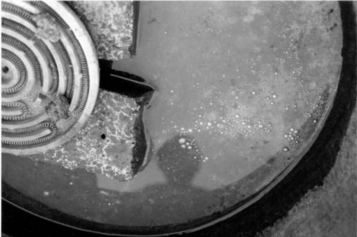
Figure 3.4 Mercury Droplets from “Gold Mountain” Retort
