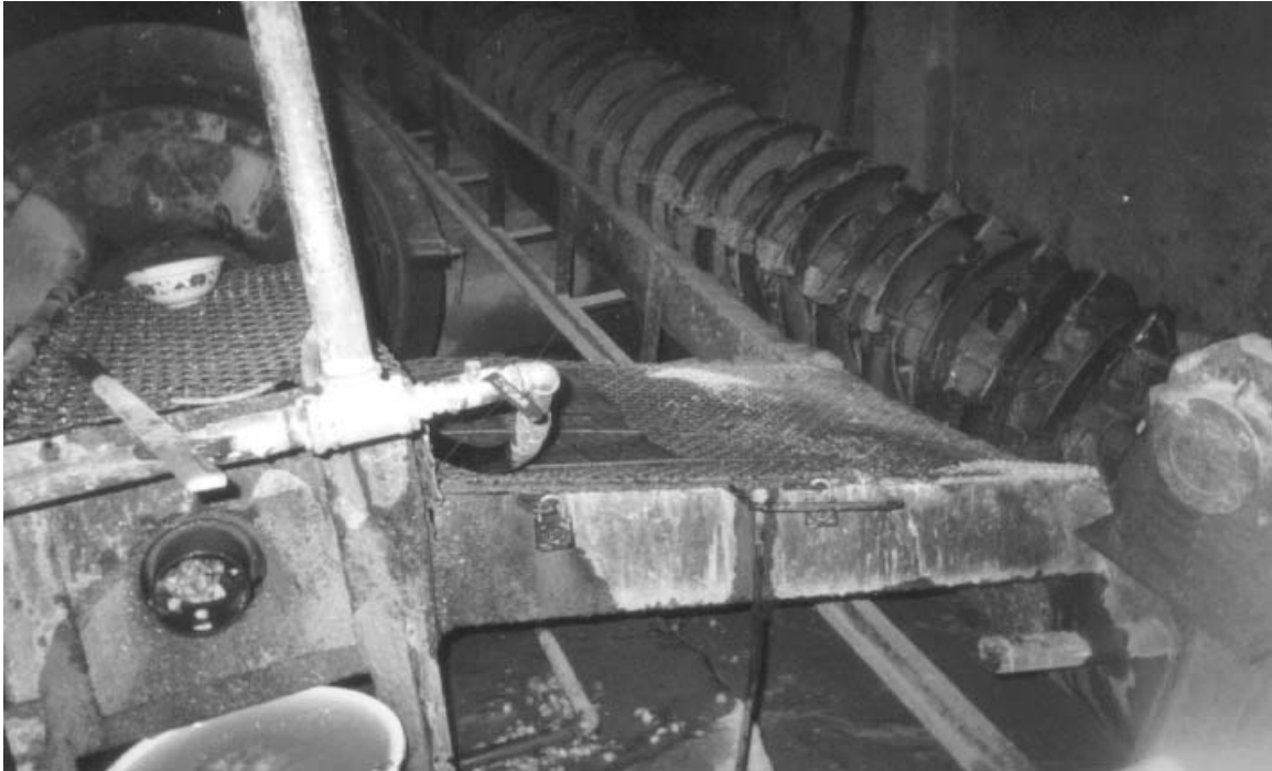
Figure 2.3 Jiangxi Ball-Mill Mercury Sluice Circuit
